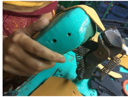
Fig: Manual Leather Pulling Tool
