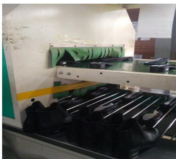
Input through heat reactivator for sole attaching
